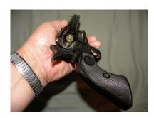
Pull hammer back to half cock, open loading gate & insert one round
