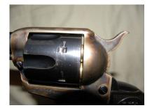
Verify that the hammer Is on an empty chamber
